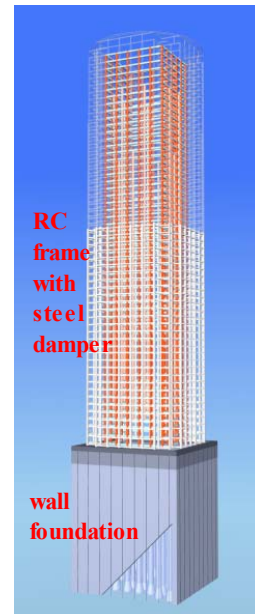
Figure 1. Skeleton view of the objective building
